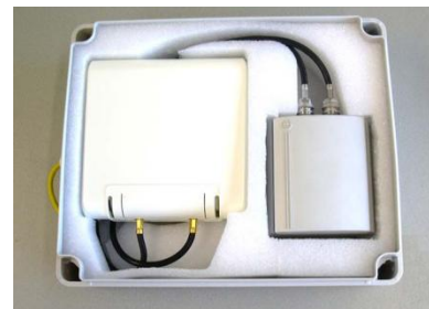
Outdoor box with AP300E and directional antenna
